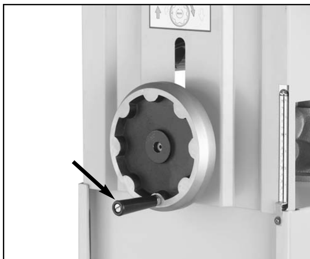
Figure 7. Install handle onto handwheel.
